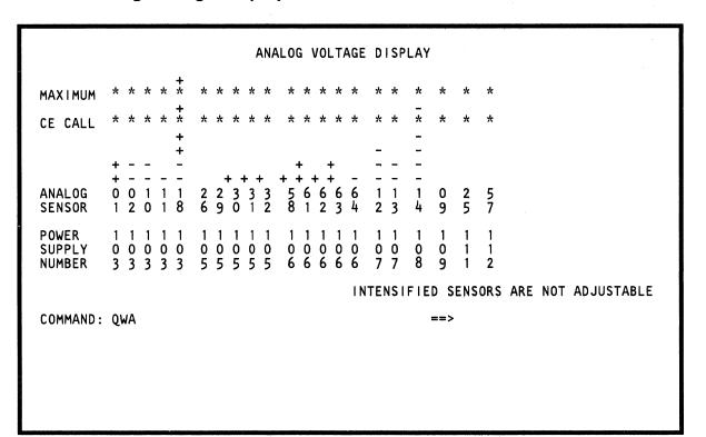
Use this screen to check that the voltage to each power supply is in tolerance.
