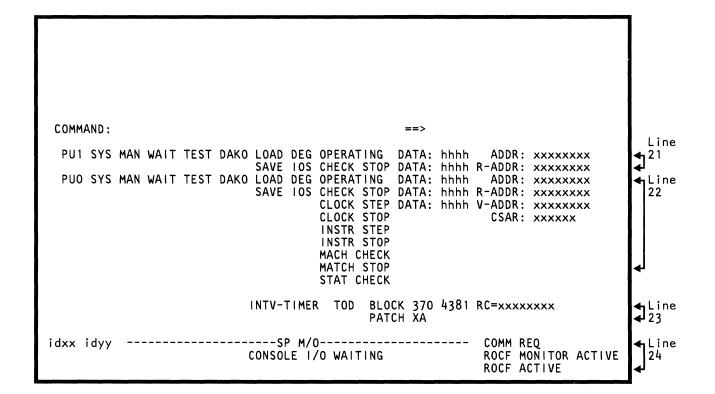
Information about the status of the system is displayed near the bottom of the display screen. A definition of each entry on the screen is given below.
