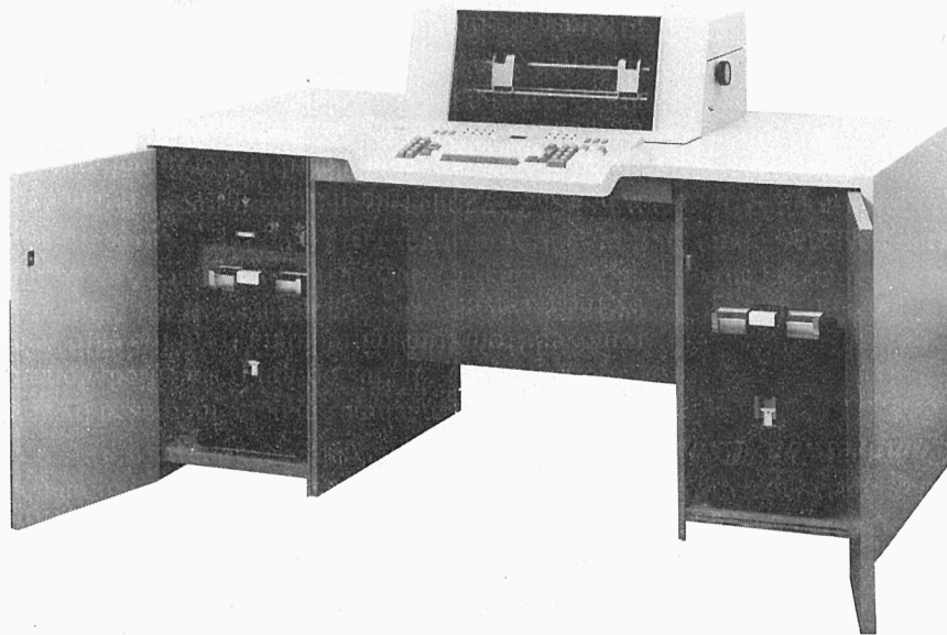
Figure 4-3. 3776 With Second Diskette Storage Device
