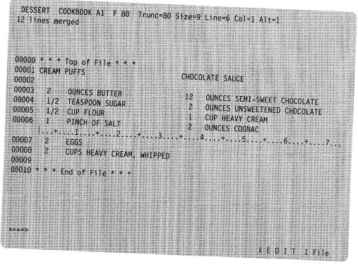
Figure 9. The MERGE Subcommand — Before and After
