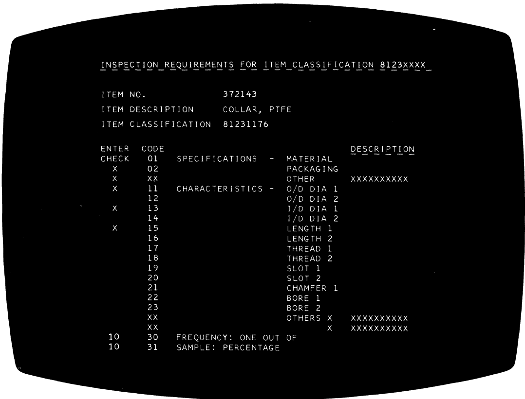
Figure 31. The quality control engineer enters inspection requirements and specifications into the system
