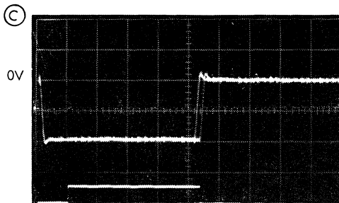
Signal Ch 1: S & H amp output A-A1A3J12 (QD891) Signal Ch 2: Same as (A)
