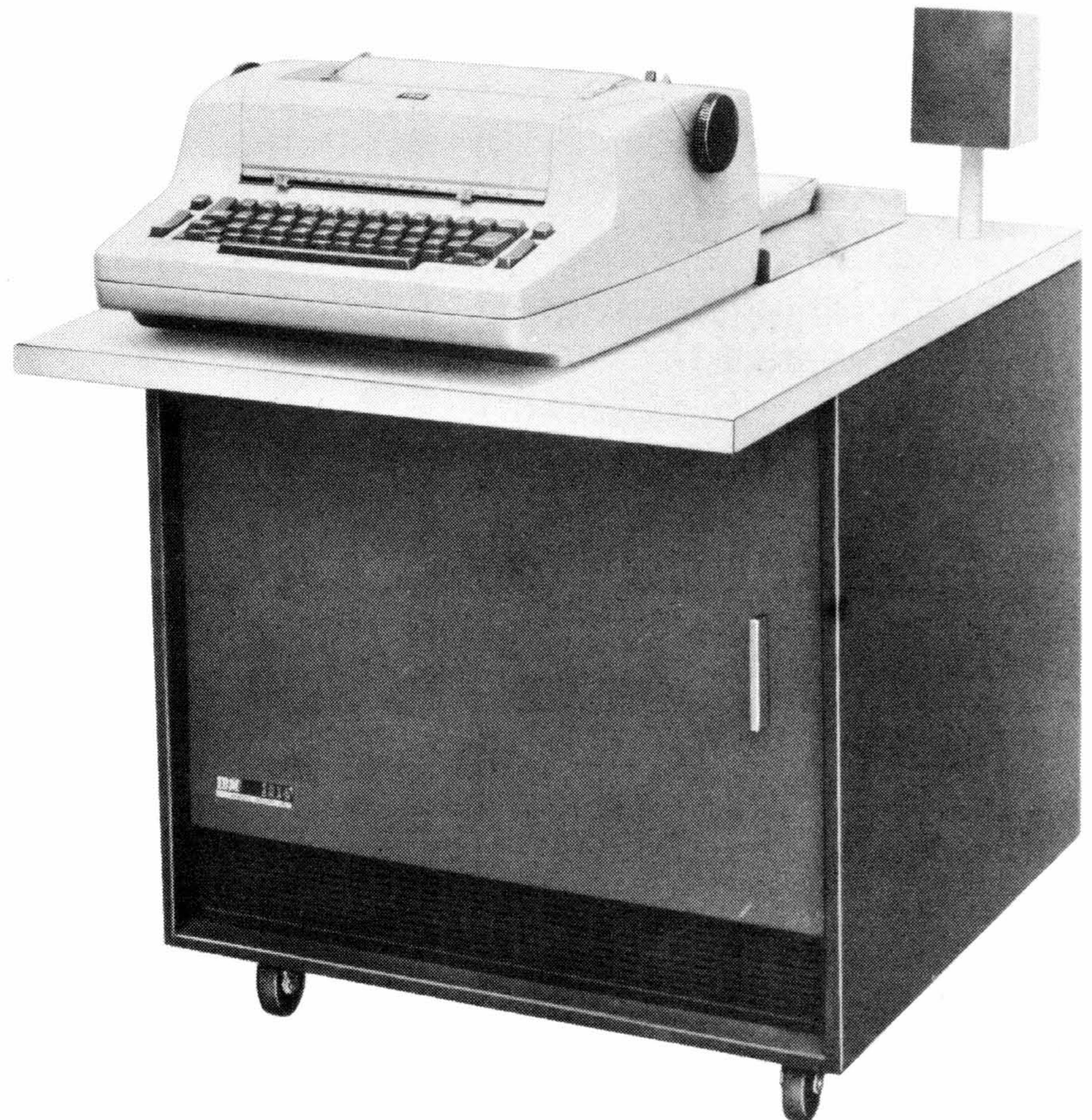
Figure 1. IBM 1014 Remote Inquiry Unit
