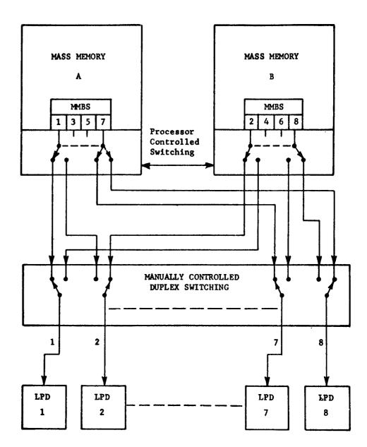
LPD's 7 & 8 are shown switched to individual channels LPD's 7 & 8 are shown switched to time share channel 7 of MMA
