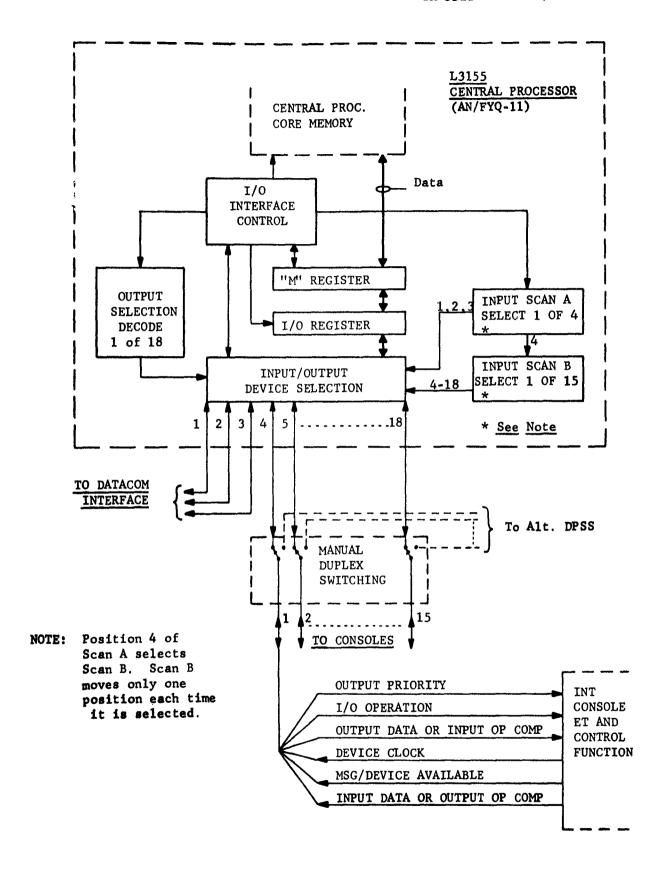
Fig. 2 ET AND CONTROL INPUT/OUTPUT INTERFACE
