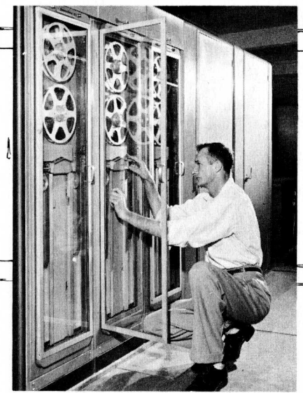
Keys to ERMA's operation are these units. Artist's conception at left shows typical input station with some of ERMA's panel boards in background. Picture at left shows one of the magnetic drums which temporarily stores activity information. In center is one of hundreds of electronic packages which do ERMA's "thinking." Magnetic tapes at right provide permanent storage of account information
