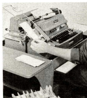
Punched cards are filed for ease of selection for insertion in Flexowriter Programatic for document preparation.
