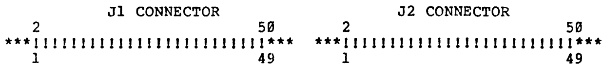
Figure 3 -- Top View of FT-68X Connectors
