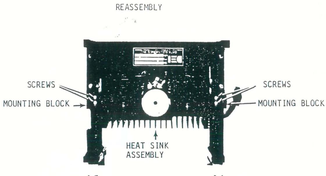
Install the Heat Sink Assembly. Pass the J701 connector through its access slot in the deck frame. Be sure to press the end of the heat sink spring into its mounting hole completely (figure 5-13). Insert the heat sink assembly into the bottom of the unit. Screw in the mounting blocks as noted above. Attach J701. Refer to 5.5.1, 2 and 3. Adjust the capstan and torsion spring. Refer to figure 5-8 and mount the Interconnect Board (or the board can be left for step 4).
