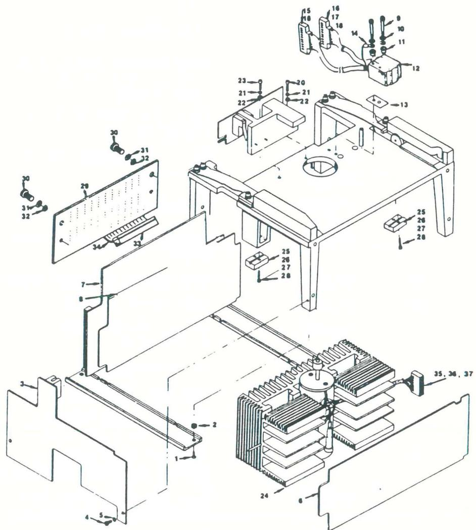
Figure 7-1. Exploded View of Drive
