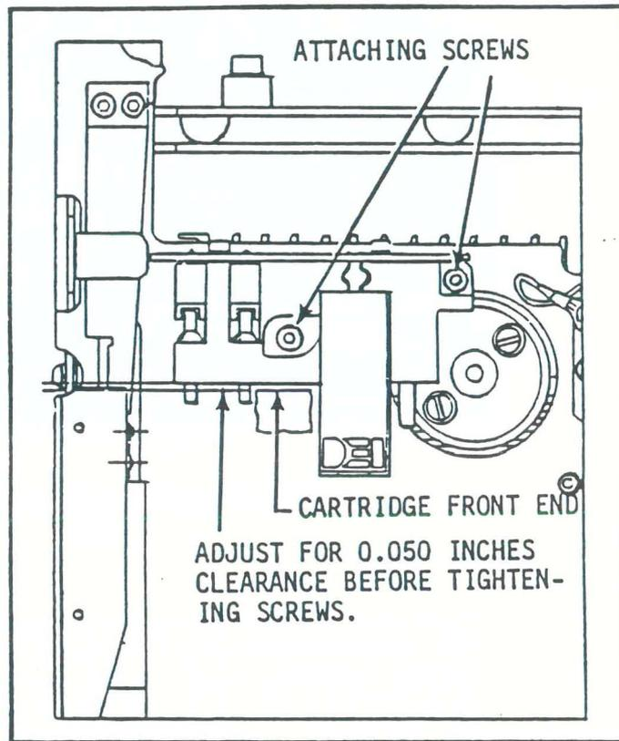
Figure 5-16. Sensor Adjustment
