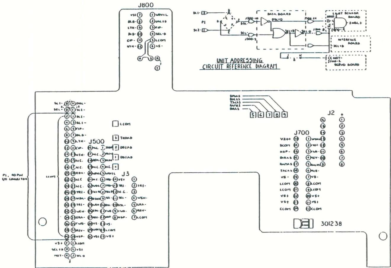
Figure 6-6. Interconnect Board, (Drive Without Control Board) 301,174
