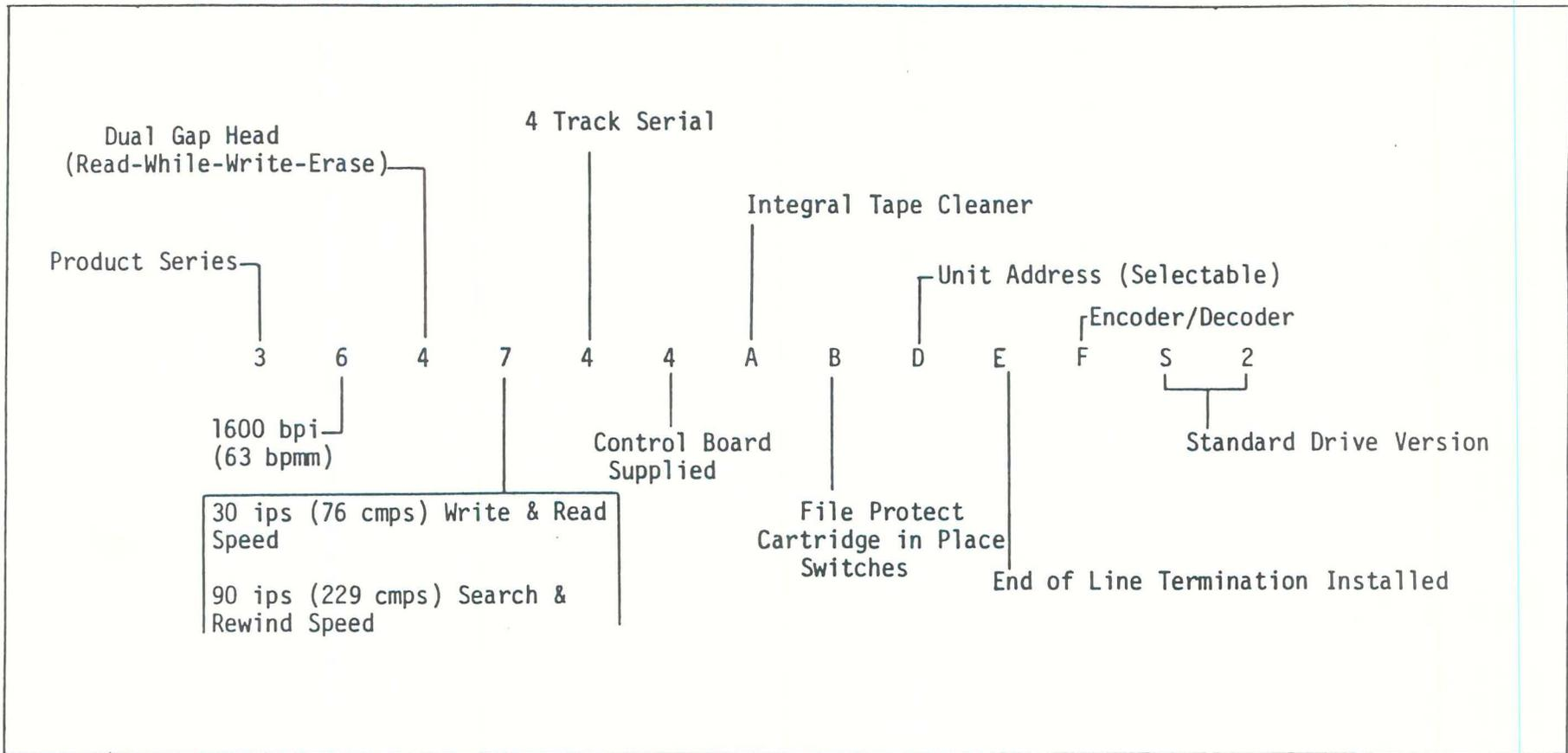
FIGURE 1-3 Model Code for Typical 1600 S2 Drive
