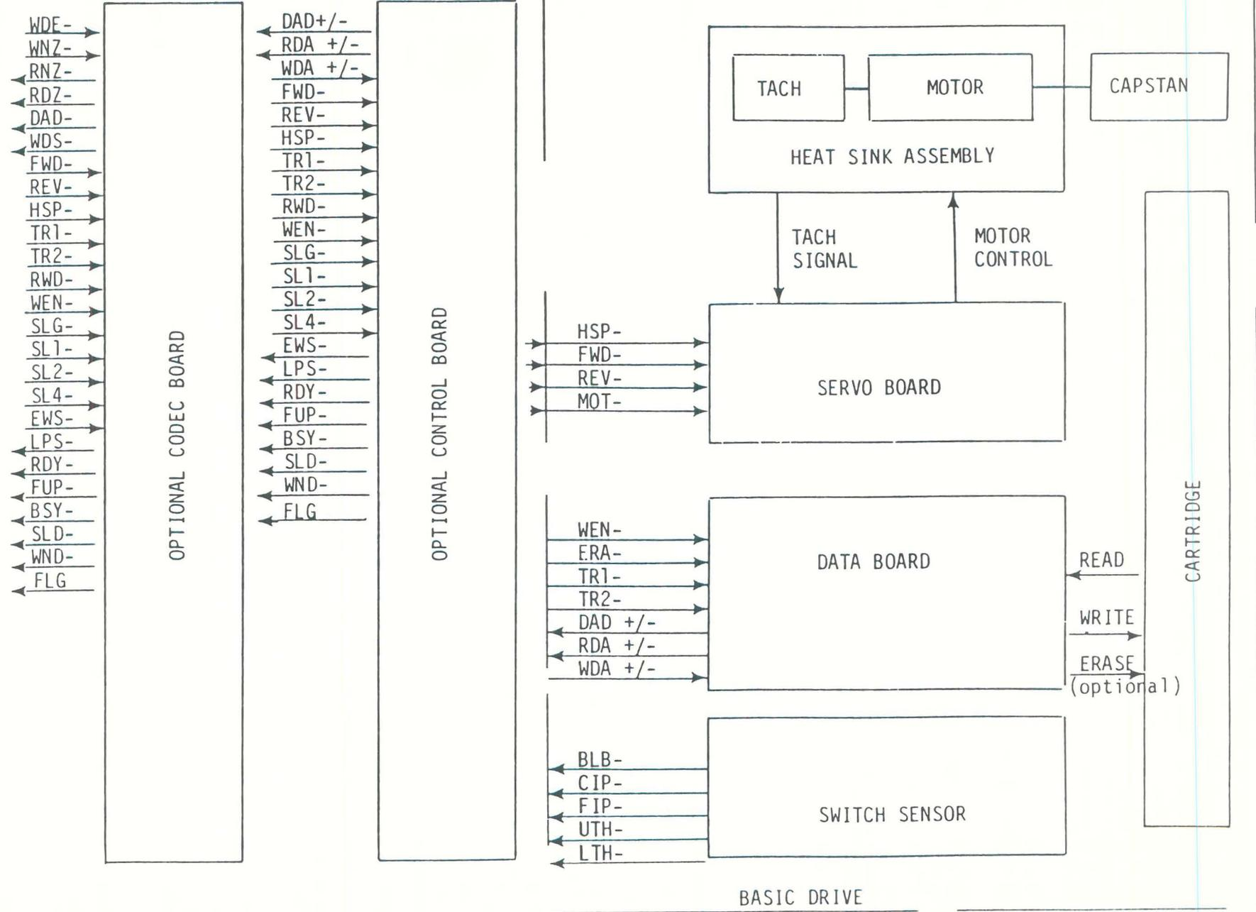
Figure 4-1. Drive Block Diagram
