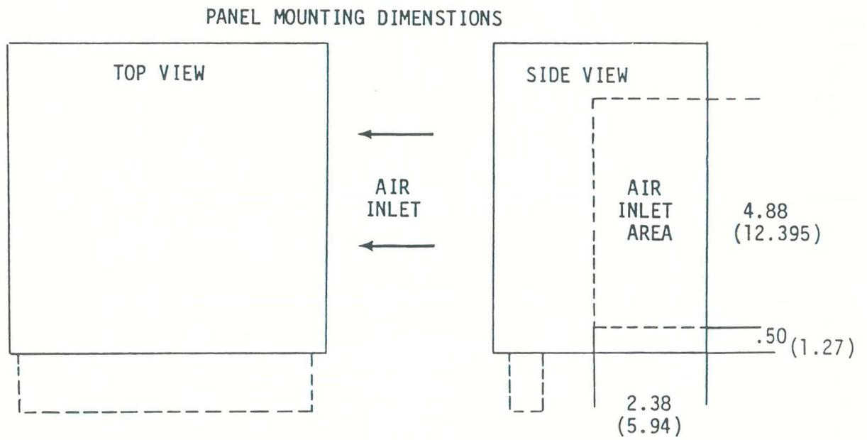
Figure 2-2. Ventilation Requirements
