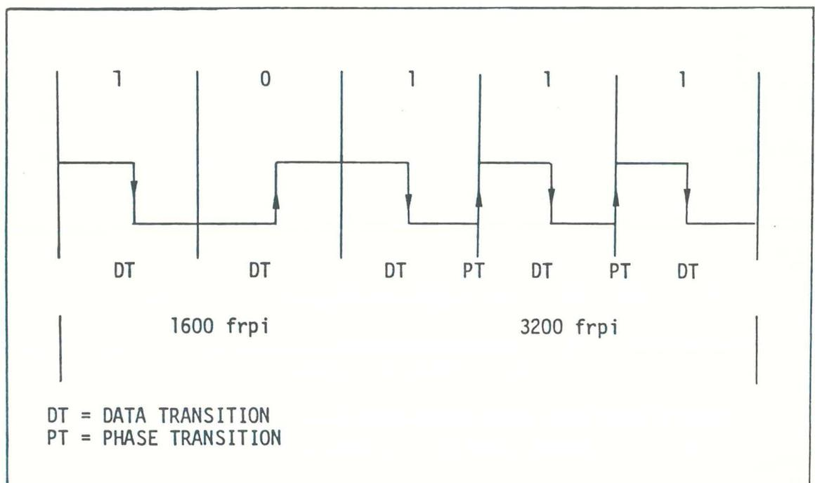
FIGURE 1-4. One & Two Frequency Waveforms
