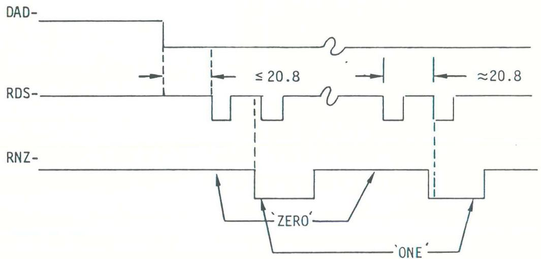
Figure 3-8. Input/Output Timing Signals for Drives with Codec Boards
