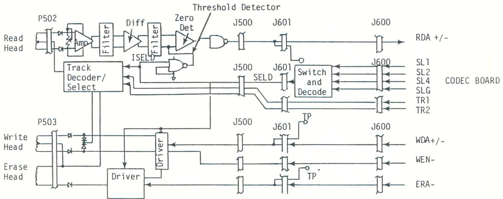
Figure 4-2. Read/Write/Erase Circuits Block Diagram (Data Board)
