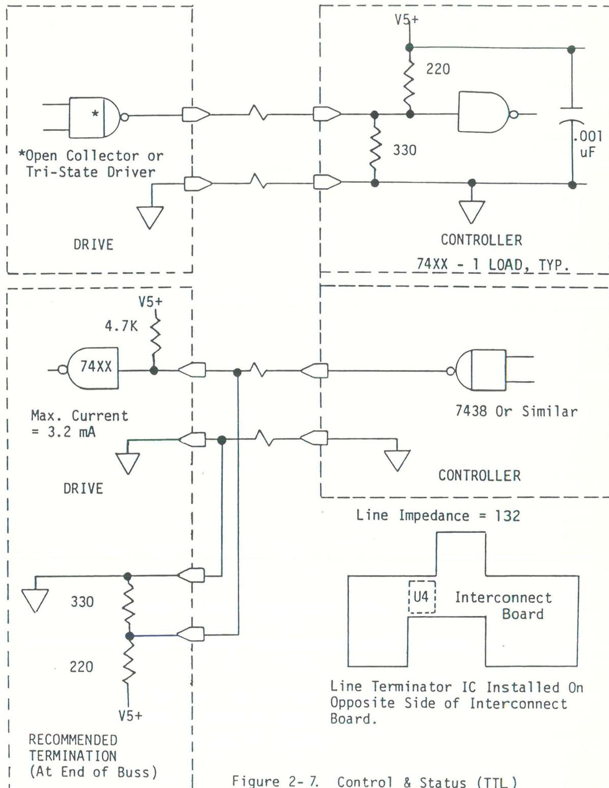
Figure 2-7. Control & Status (TTL) Signal Termination
