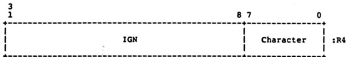
Figure 8-8: Console Transmit Data Buffer Register (CTDB)
