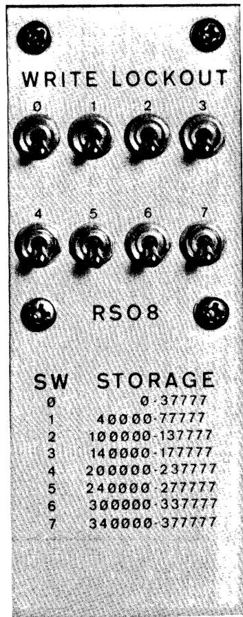
Figure 4-1 Write Lockout Switch Diagram
