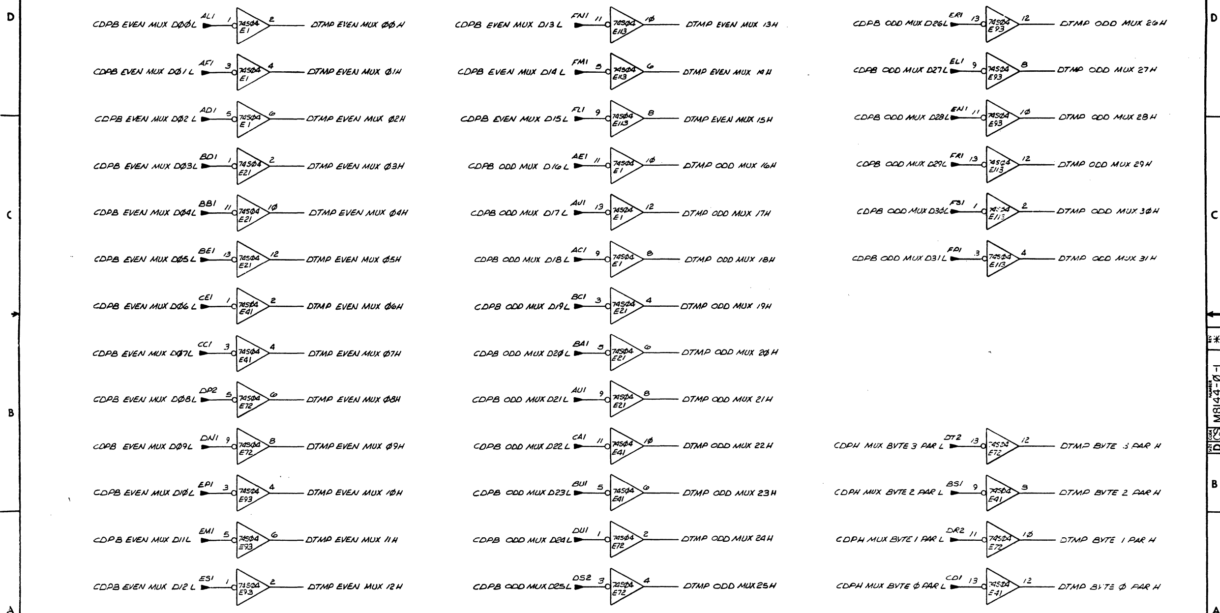
SLOT 20 (MAIN MEMORY DATA INVERTERS)
