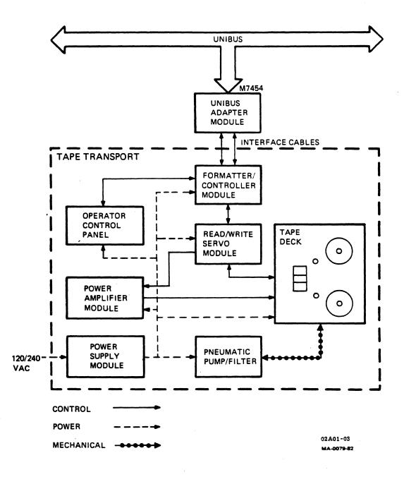
Figure 1-2. TU80 TAPE SUBSYSTEM BLOCK DIAGRAM
