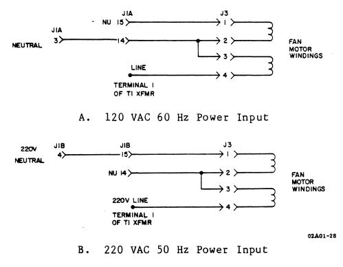
Figure 4-5. COOLING FAN WIRING
