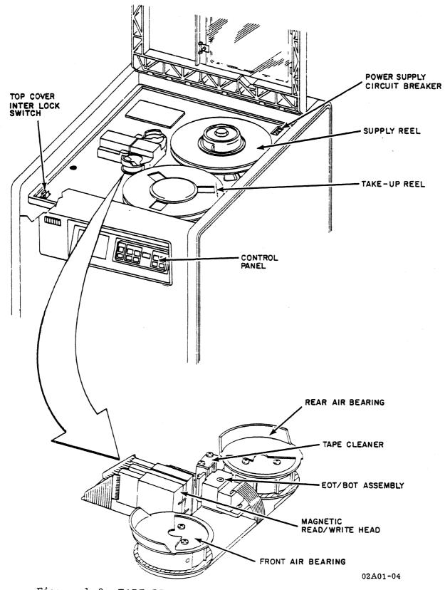
Figure 1-3. TAPE DECK COMPONENT LOCATIONS, TOP VIEW
