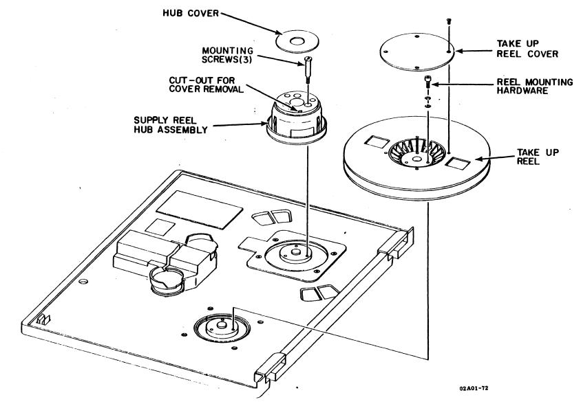
Figure 5-6. Take-Up Reel/Supply Hub Assemblies
