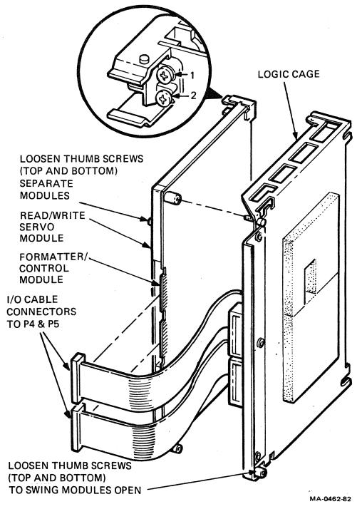
Figure 5-24. LOGIC MODULE REMOVAL/REPLACEMENT
