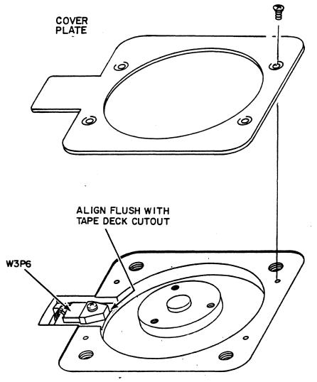
Figure 5-4. FILE PROTECT SENSOR ALIGNMENT
