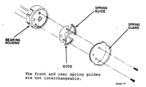
Figure 5-11. AIR BEARING SPRING GUIDE
