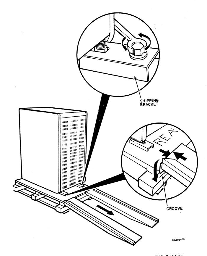
Figure 2-3. REMOVING THE TU80 FROM SHIPPING PALLET
