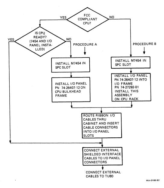
Figure 2-13. I/O CABLING FLOWCHART
