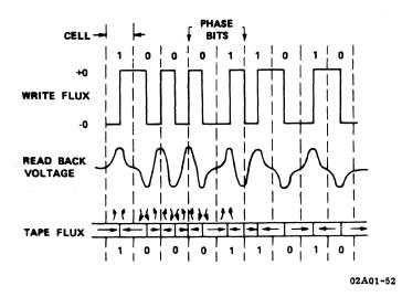
Figure 4-30. PE MODULATION RECORDING
