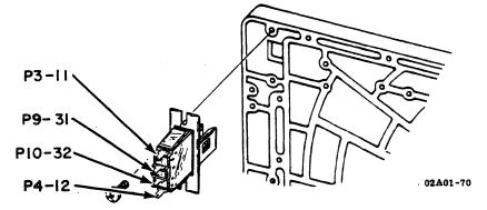
Figure 5-3. TOP COVER INTERLOCK SWITCH (MAINTENANCE VIEW)
