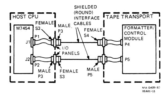
Figure 2-10. PLUG-TO-PLUG INTERFACE CABLE CONNECTIONS
