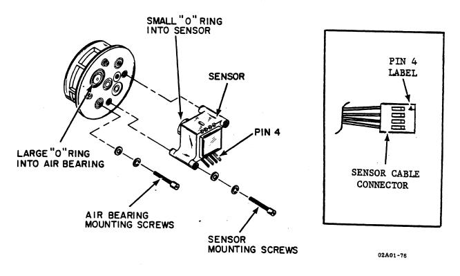
Figure 5-10. AIR BEARING SENSORS
