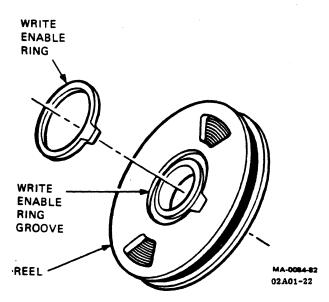
Figure 3-2. WRITE ENABLE RING
