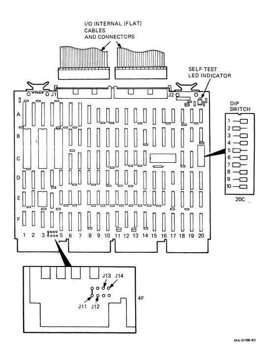
Figure 2-11. DIP SWITCH ON M7454 MODULE
