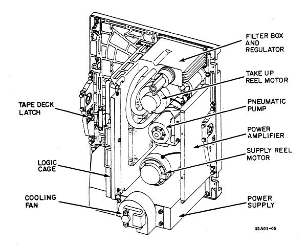
Figure 1-4. TAPE DECK COMPONENT LOCATIONS, REAR VIEW (ACOUSTIC COVER REMOVED)
