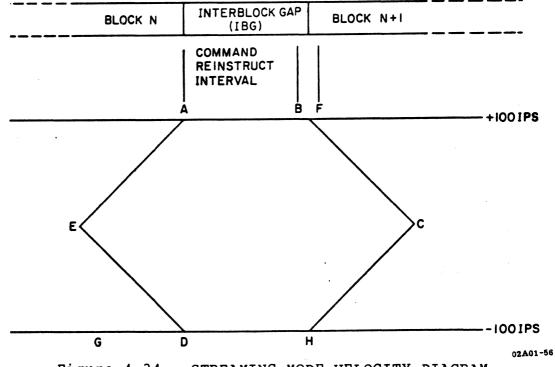
Figure 4-34. STREAMING MODE VELOCITY DIAGRAM
