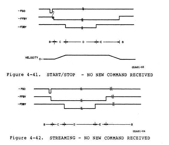
State E - This state is the reinstruct interval. Receipt of a follow-up command identical to the previous -FGO command continues tape motion at either low or high speed in streaming mode. Refer to Figures 4-40 and 4-44.
