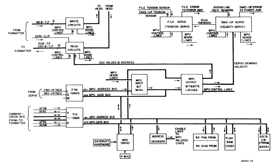
Figure 4-12. READ/WRITE/SERVO MODULE BLOCK DIAGRAM
