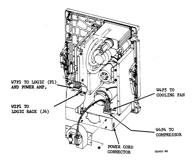
Figure 5-19. POWER SUPPLY CONNECTORS
