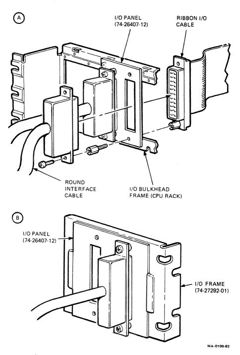
Figure 2-14. I/O CABLE INSTALLATION
