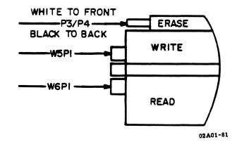
Figure 5-15. MAGNETIC HEAD CONNECTORS
