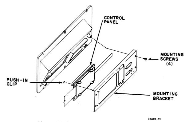
Figure 5-17. OPERATOR PANEL ASSEMBLY
