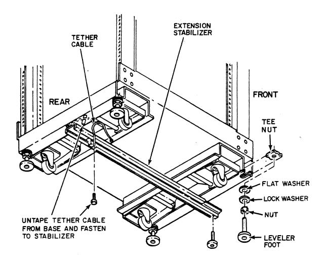
Figure 2-4. CABINET LEVELER FEET ASSEMBLY AND EXTENSION STABILIZER
