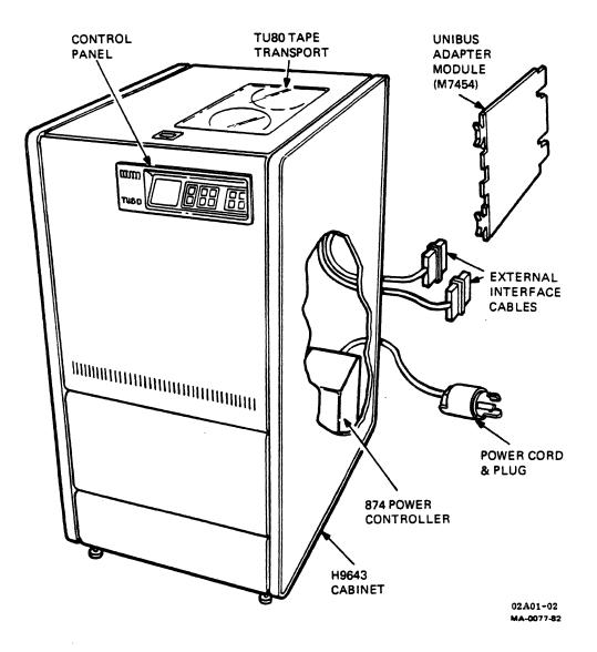
Figure 1-1. TU80 TAPE SUBSYSTEM
