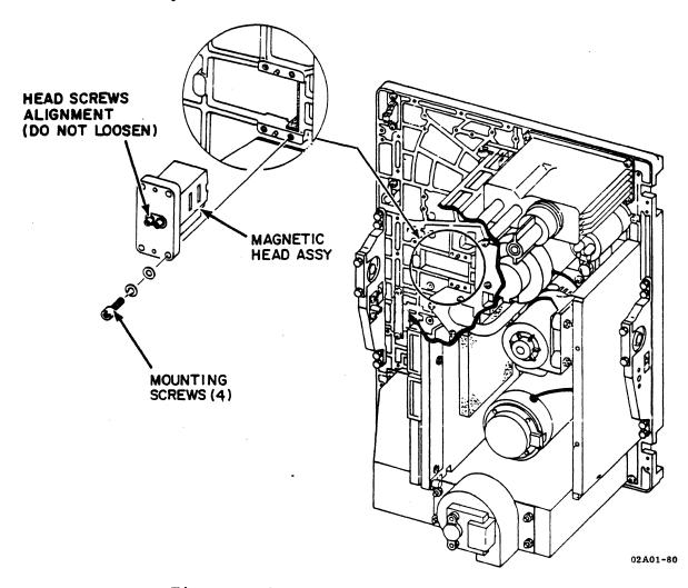
Figure 5-14. MAGNETIC HEAD ASSEMBLY
