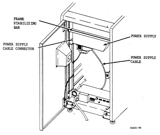
Figure 5-20. POWER SUPPLY (REAR CABINET VIEW)
