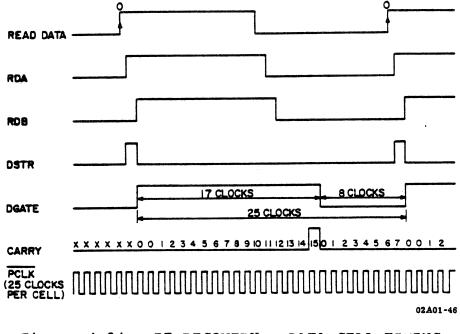
Figure 4-24. PE RECOVERY - DATA CELL TIMING
