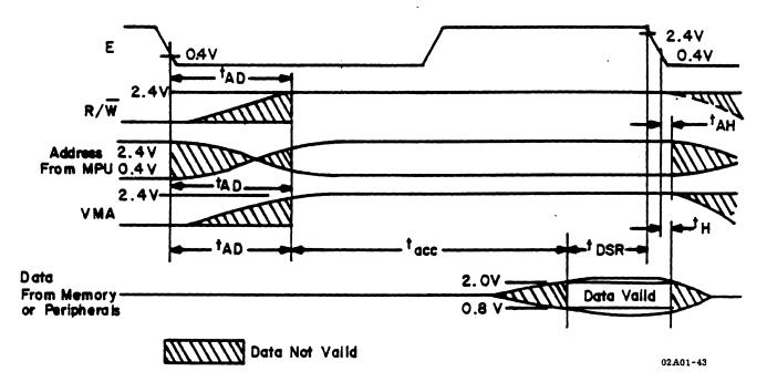
Figure 4-21. PROCESSOR READ OPERATION
