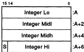
A quadword integer operand occupies 64 bits in a floating register, arranged as shown in Figure 2-18.
