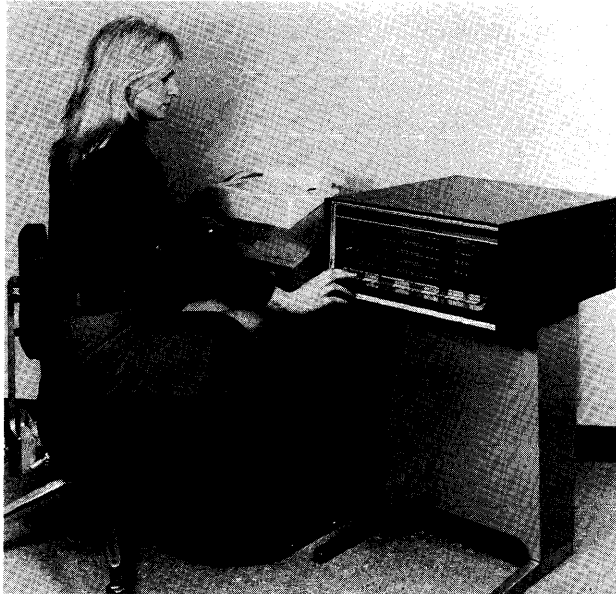
Digital Computer Controls caused a stir in the minicomputer world by building machines that offer both plug and program compatibility with the popular DEC PDP-8 and Data General Nova computers. The D-112 shown here is a direct replacement for the PDP-8, while the D-112H offers higher speeds and an expanded instruction set.
