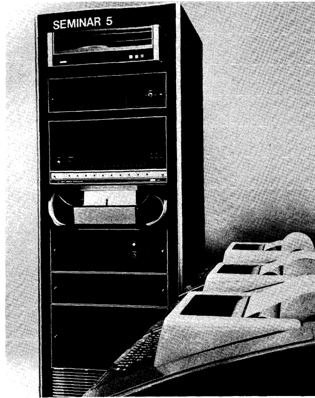
Data General's SEMINAR 5 time-sharing system, based upon a 24K Nova 800 minicomputer with both fixed-head and moving-head disk storage units, can serve up to 16 simultaneous users at remote teletypewriters. Designed for high schools and colleges, it exemplifies the "packaged" systems that the larger minicomputer builders are developing to increase their penetration of end-user markets.
