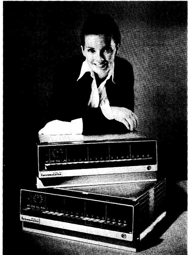
The first two members of Interdata's "New Series" exemplify many of the current trends in minicomputer design. Model 70 (bottom) uses a 1-microsecond core memory, while the faster Model 80 employs a 240-nanosecond MOS main memory. Both models utilize LSI circuits and are controlled by microprograms in fast bipolar read-only memories.
