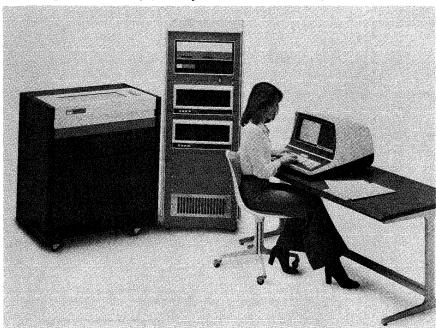
The BDS Series 2000 basic system includes a processor with 32K bytes of memory, two 10-megabyte disk drives, an 8-channel I/O interface, one CRT, and a 300-lpm line printer. The purchase price is \$63,089.
