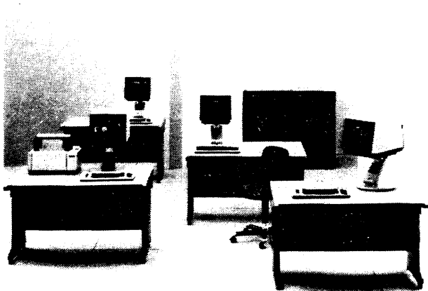
The 8850/50 configuration shown is based on one of five 8850 models available, and can support up to 32 workstations, one 16MB fixed disk, and four diskettes.
