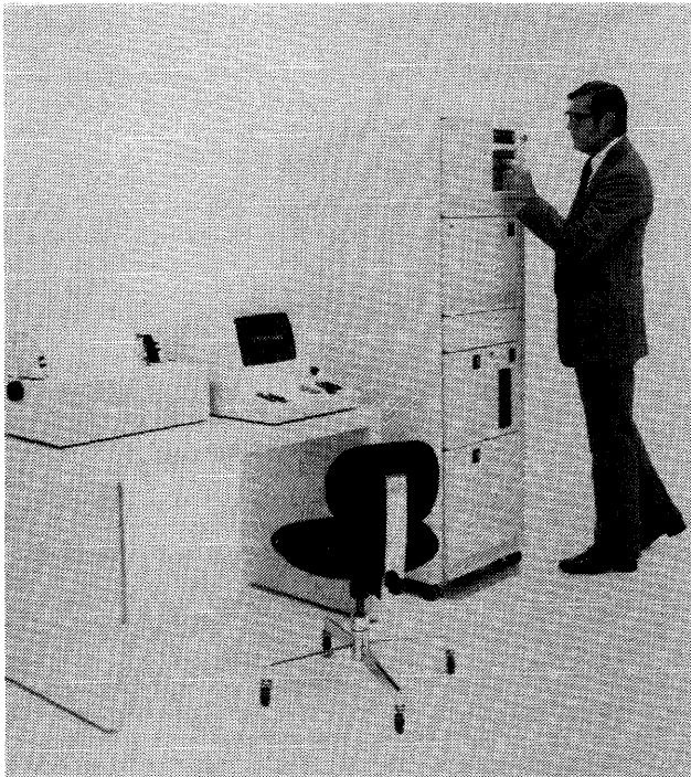
The Series/1 Model 5 system shown here includes a 9.3-million-byte disk subsystem with a built-in 492,000-byte diskette unit. The 120-cps printer and the display station with a 1920-character CRT screen are shown at left.
