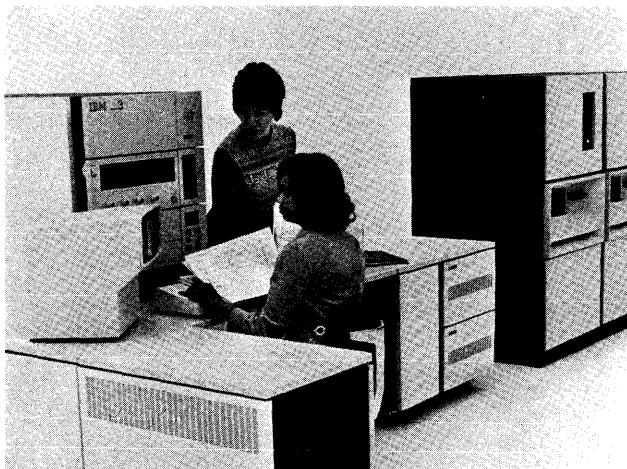
The Model 15 CPU features an operator console with CRT display output and keyboard input. At right are two 5445 Disk Storage Drives, which use interchangeable 2316 Disk Packs and can store 20.48 million bytes each.
