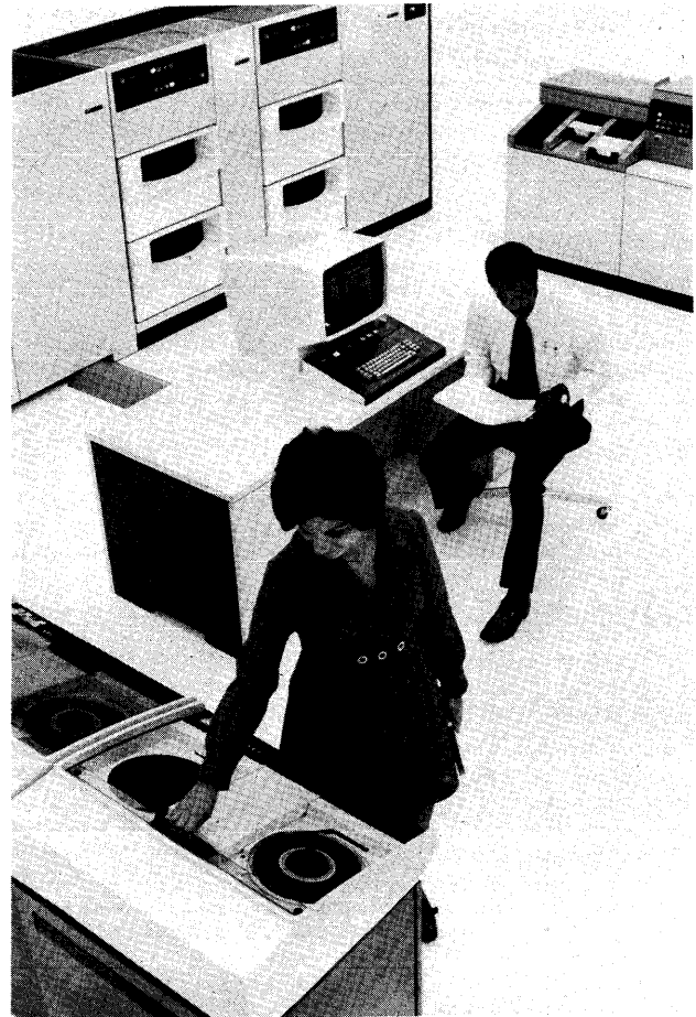
The Model 125, introduced in October 1972, was the first IBM system below the "super-computer" class to employ distributed processing techniques. Direct access storage devices available for the Model 125 include the 3330 Series Disk Storage drives (left rear) and the newer 3340 Direct Access Storage Facility.
