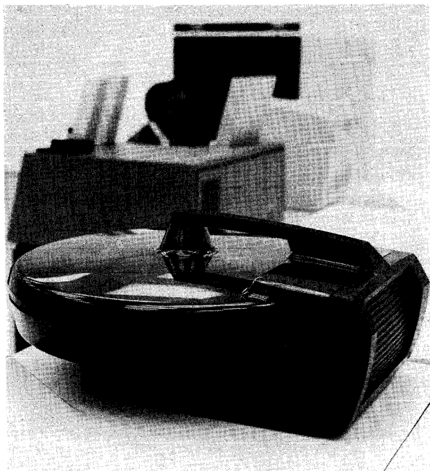
Weighing in at 16 or 18 pounds, the two models of IBM's new 3348 Data Module store up to 35 million or 70 million bytes of data, respectively, and combine the disks, access arms, and read/write heads into a single sealed cartridge.
