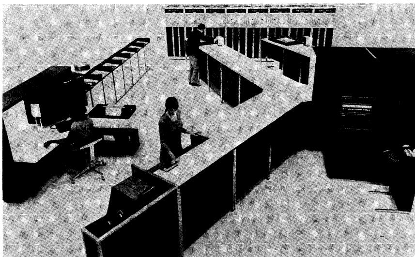
This Model 2060 tape/disk system, arranged in a distinctive Y-shaped configuration, is equipped for multiprogramming and communications processing. The Visual Information Control Console is at the far left and the DATANET 2000 Communications Processor at the far right.
