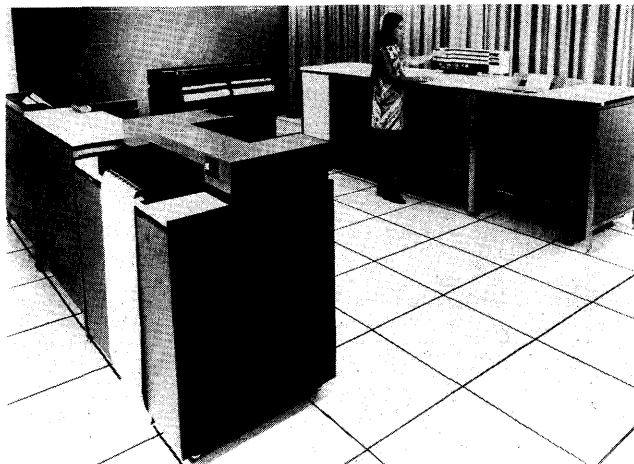
Smallest member of the Series 200/2000 family, the Model 105 system can be rented for less than $2,000 per month. A Model 105 system can include up to 9.2 million characters of disk storage and can process programs written in COBOL, FORTRAN, and RPG.
