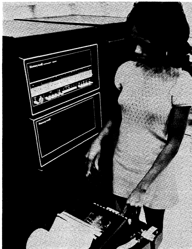
The DATANET 2000, introduced with the Series 2000 computers, is a minicomputer-based front-end processor that controls up to 120 lines and significantly improves the data communications capabilities of the medium-scale Honeywell computer systems.
