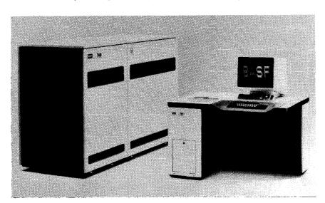
The BASF 7/68, a plug-compatible substitute for the IBM 4341-2, is based on the Hitachi M240H and can support both IBM and BASF peripherals. BASF reports that tests show the 7/68 is about twice as fast as the 4341-2 while taking up less space and generating less heat.
