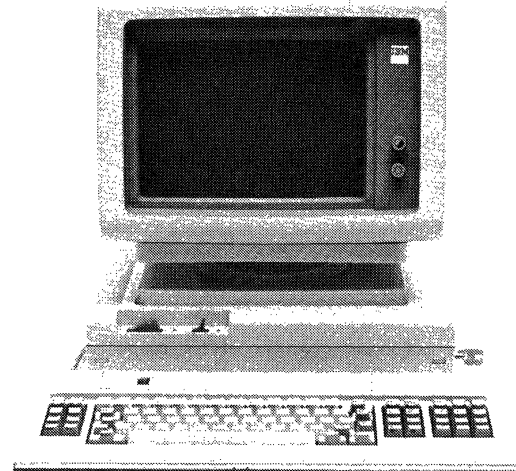
The IBM 3178 Display Station is a small-screen, small-footprint version of the successful 3278 Model 2. Several independent 3270-compatible vendors have already introduced competitive models.
