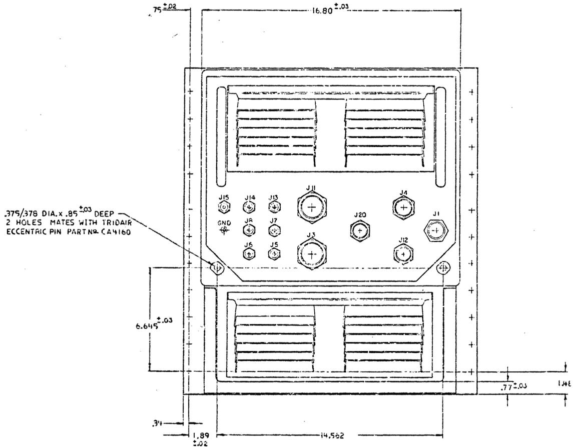
Figure 3-6. Outline and Installation Display Driver Assembly
