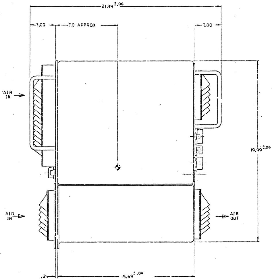
Figure 3-6. Outline and Installation Display Driver Assembly
