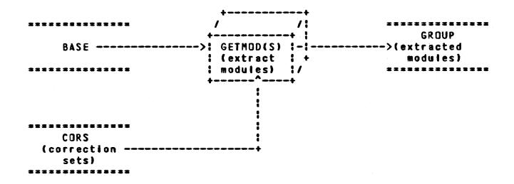
GETMOD(S) is a fairly simple process: a list of modules is extracted from the base library, and appear on file group in MADIFY source form, that is, one module per logical record. An optional correction set (the cors parameter) may be applied temporarily to the base before the modules are extracted. Procedure TEMPCOR applies the temporary correction sets.
