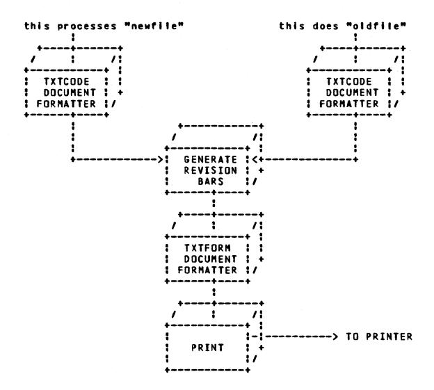
This diagram shows the action taken when you run FORMAT with a current document and a "base" version of the document. The revision bar generator compares the two files after TXTCODE has processed them, and generates the commands such that TXTFORM knows where to place revision bars in the final document.
