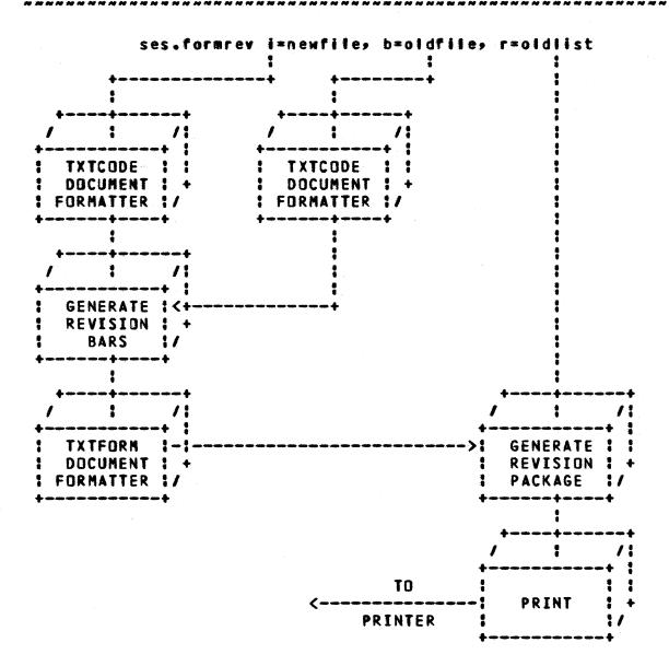
This diagram shows FORMREV used to generate a revision package where all three forms of the document are used: the current version of the document, newfile, the old version of the document source, oldfile, and the old document listing, oldlist. In this case, FORMREV uses the old listing as the base against which to compare the processed version of the new document. Because the old document source was used as well, the change pages produced by FORMREV have revision bars on them.
