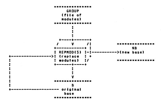
REPMOD(S) takes modules from a group file (which, as shown in the diagram, could well have come from the old base in the first place), and replaces (or adds) them to produce either a completely new base, or rewrites the result over the old base.
