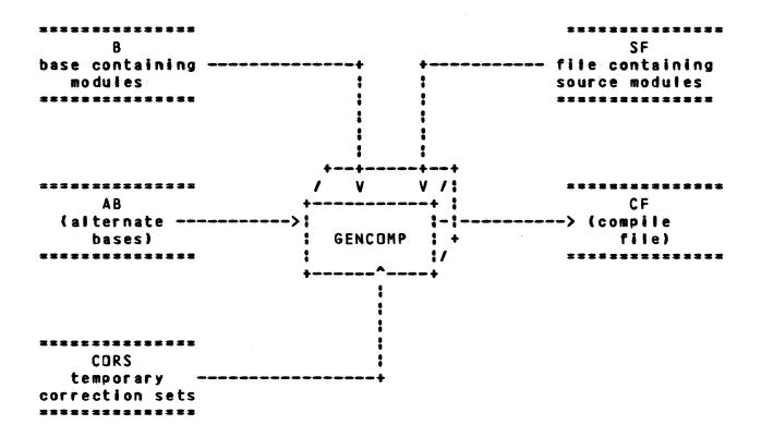
GENCOMP generates a compile file for modules which may come from off the base (the m parameter), or from a source file (the sf parameter), or from both places. The ab parameter specifies a list of alternate bases to be used to get common decks from. A temporary correction set may be applied (the cors parameter) via the TEMPCOR procedure before generating the compile file.
