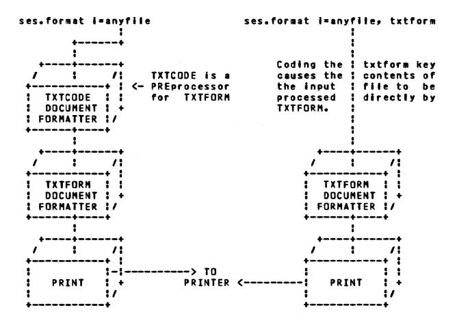
The diagram shows two of the ways that FORMAT can run, depending on the options you code. The left hand diagram shows the normal and simplest case of FORMAT. The right hand diagram shows that coding the txtform or form key eliminates the TXTCODE process.
