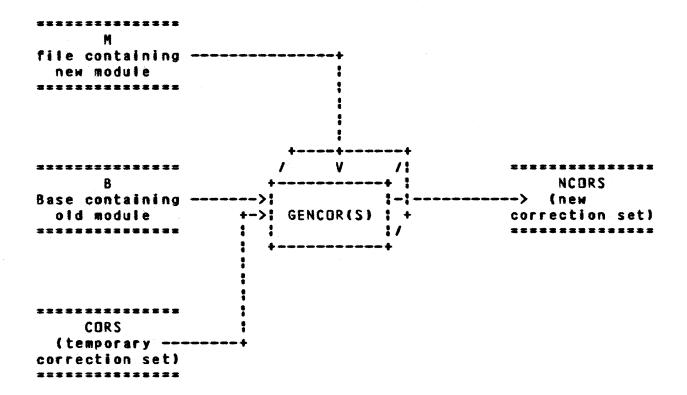
The picture shows the flow of GENCOR(S). The file containing the new module M is in the user's catalog. The old version of the module is in the base B. An optional temporary correction set (CORS) may be applied if desired, in which case GENCOR(S) uses the TEMPCOR procedure to apply the correction set before generating the new correction set, which appears on the file specified by the ncors parameter.
