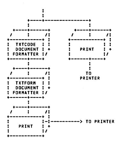
This diagram shows what happens when you run FORMAT and code the source key. The source of the document is printed directly, then the formatting process takes place to produce a formatted document.
