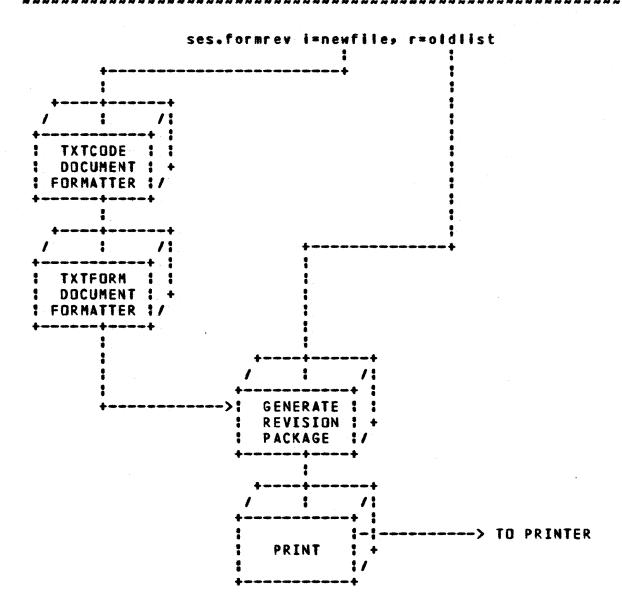
This diagram shows the simplest use of FORMREV. The current version of the document is compared with the old listing of the document in order to generate a change package. In this case there are no revision bars generated on the final output since there was no old document source given to FORMREV to be processed.
