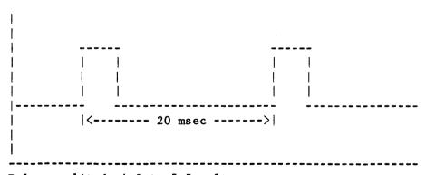
Pulse amplitude 4.5 to 5.5 volts
