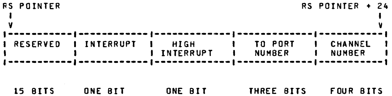
Figure 3.6 Result Descriptor - Single-Line Control
