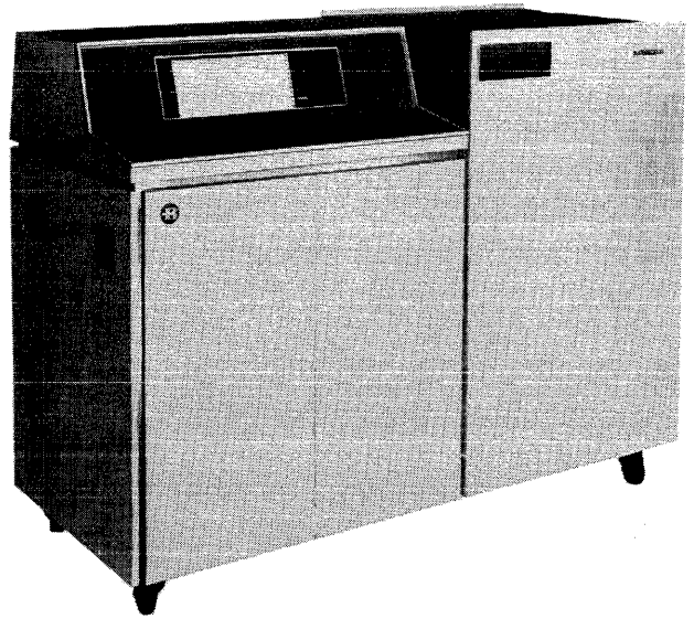
Figure 2-43. B 321 Line Printer
