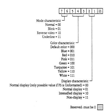
Fig 1-3 1-2-B (L02) Basic DAB byte format Zoro
