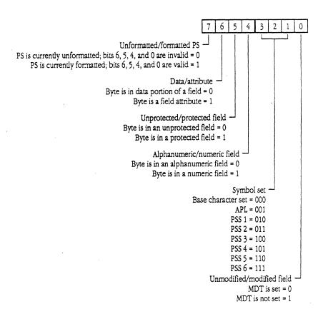
Fig. 1-4 1-3-B (L03) Extended DAB byte Zoro
