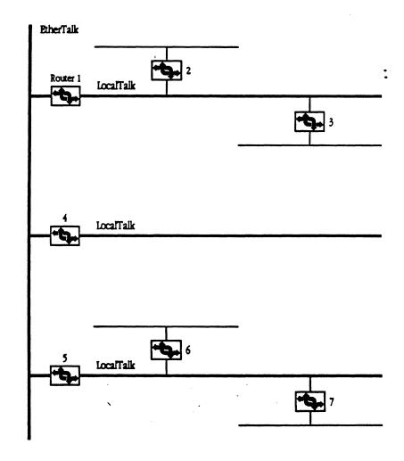
2. To begin, upgrade Router 1 to an AppleTalk Phase 2 router and install the Upgrade Utility.
