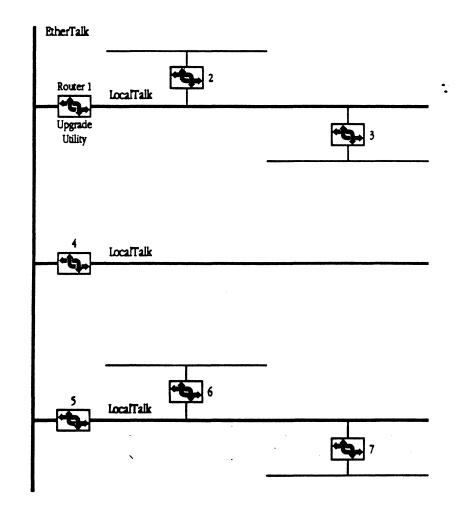
3. Once Router 1 has been upgraded and the Upgrade Utility installed, upgrade Router 2 and Router 3. Since routers 2 and 3 are connected to a LocalTalk network, they must either be upgraded at once or upgraded using the Upgrade Utility.
