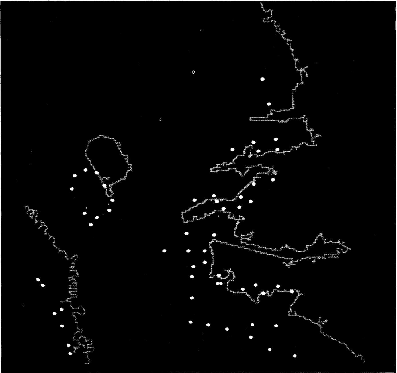
Figure 4—Predicted image coordinates of coastline (based on navigational estimates of camera location and orientation) superimposed on extracted boundary.
