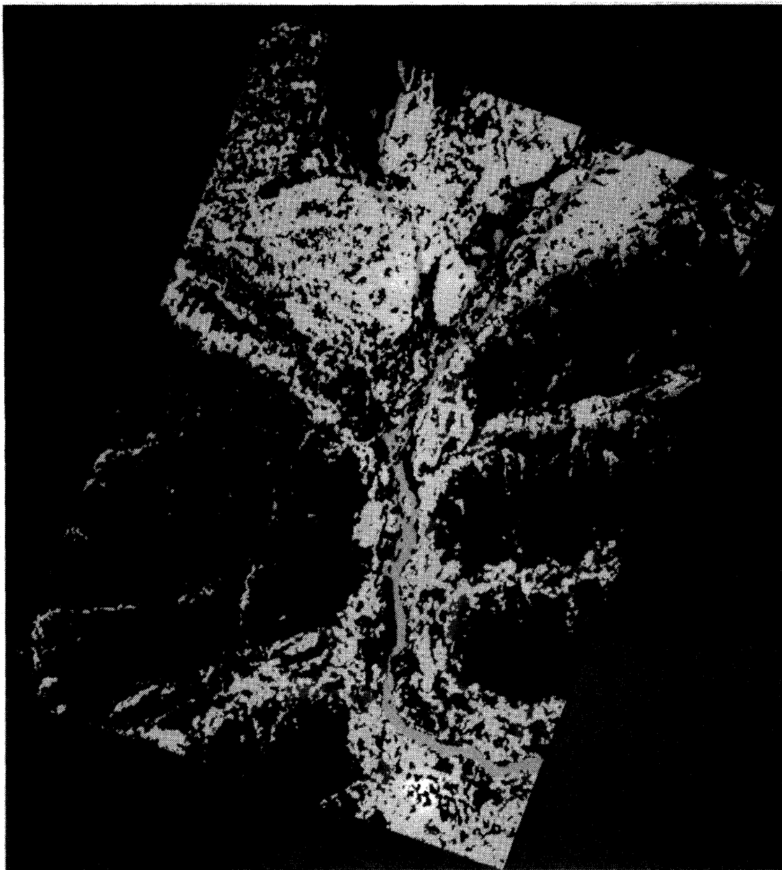
Figure 11.—Landsat classification of land cover types near Cantwell, Alaska. A spatial smoothing algorithm was used to eliminate the "Salt-and-pepper" appearance as shown in figure 5. The smoothing was done to simulate an approximate four ha (ten ac) minimum mapping unit. Barren lands are shown in black. Clear water and sediment laden rivers are shown in dark green; low shrub is shown in light green, and tall shrub is shown in red. Open conifer—tall shrub is shown in light red; open conifer—low shrub is shown in violet, and dense conifer is shown in purple.
