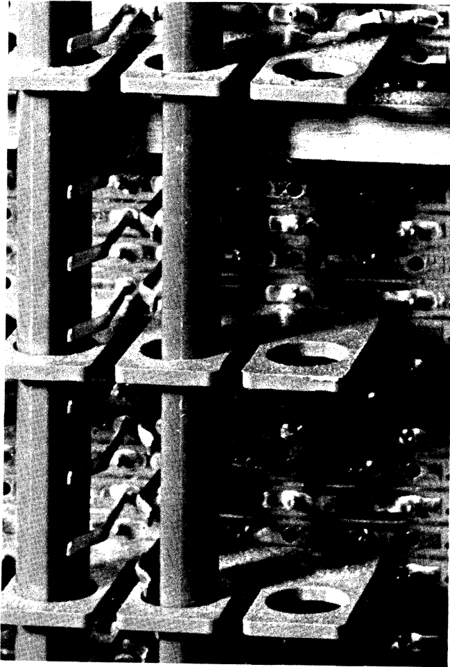
Figure 6—Zero insertion force, cam-operated connector system
