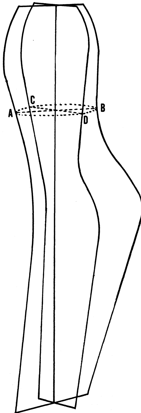
Figure 6—Diagram showing how the computer uses the PROSA input mode to combine 4 profiles and from them derive a contour slice AD BC. 48 of these sections are stacked on the vertical axis to define a complete form. It can be seen that if the same profile were to be used in all positions ( +X and -X , and +Y and -Y ) the form would have radial symmetry and all the sections would be circles. Available as options are yet other systems of symmetry
