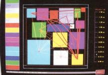
High complexity Cell-Based ASICs require advanced tools like the MDE chip floorplanner to optimize delays and verify performance prior to layout.
