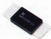
The original BiCMOS 256Kx1 at 15 ns
