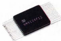
The new BiCMOS 64Kx4 at 12 ns
