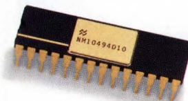
The new BiCMOS 16Kx4 at 10 ns
