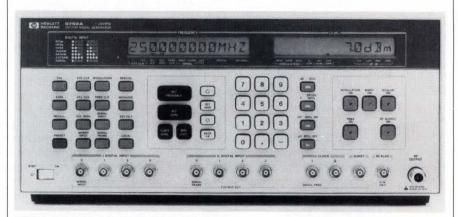
2. SEVERAL FORMS of digital modulation, including 256 levels of quadrature amplitude modulation (QAM) and 81 levels of pseudo-random-sequence (PRS) modulation, are available from the HP 8782A vector signal generator.
