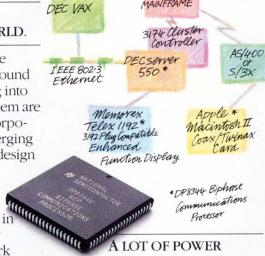
An intelligent transceiver and high-performance CPU are integrated on the same low-power CMOS chip. So a full system supporting all three IBM protocols—3270, 3299 and 5250—can be implemented in an area the size of a credit card.
