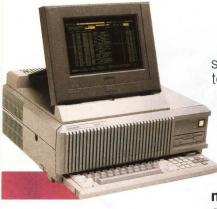
The Prism 3002P configuration features a slide-away keyboard and a 640x400 flat panel display that folds against the mainframe when not in use.
