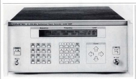
1. A TWO-LINE DOT-MATRIX alphanumeric display on the Wavetek 2407 includes instructions for operating the unit's extensive set of built-in diagnostic and calibration routines.
