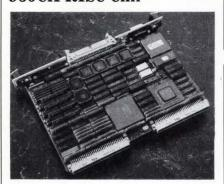
argeted at real-time control applications such as communications and image processing, a VMEbus board from Heurikon Corp. is the first to use Intel's new 960CA RISC chip. In addition to the processor, the HK80/V960E board features on-board SCSI and Ethernet interfaces, and zero-wait-state memory access.
