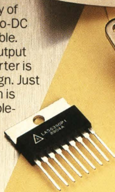
DC-TO-DC STEP-DOWN CONVERTER 1,2
