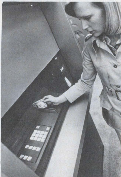
Bank cash terminals , such as IBM's 3614, dispense money after a verified user inserts a cash card.
