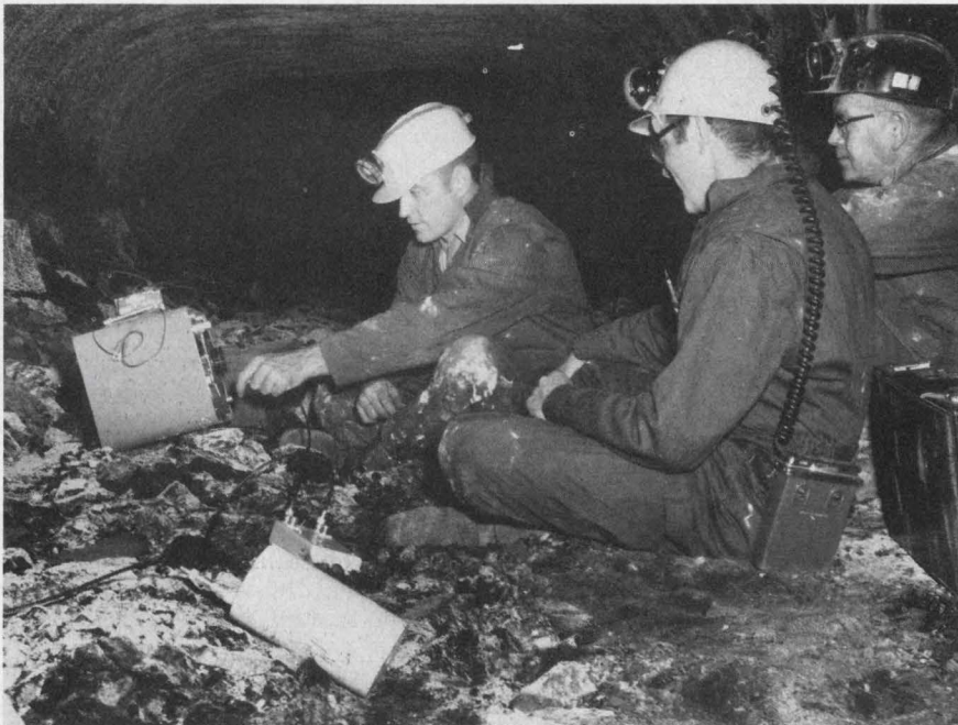
Underground field strength measurements are being made by Westinghouse engineers in the Eagle Coal Mine in Colorado. Evaluation of the penetration depth of ulf radio transmissions was aided by these measurements.
