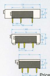
A full watt in less space — You can increase both part density and power handling ability with either the 2700 (wirewound) or 8700 (cermet) series. Both dissipate one watt at 70° C.
