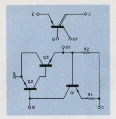
A new symbol (top) has been proposed by Mitsumi for the Semicon L device. Equivalent circuit is shown beneath it.
