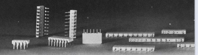
You name it—we have the exact cermet resistor network size and characteristics you need. Here's the choice you get right now: our 750 line includes: .100" centers with 4, 6 & 8 pins; .125" centers with 2, 4, 6 & 8 pins; and .150" centers with 4 through 13 pins. And we're working on new designs right now!
