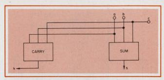
3. Block diagram of a conventional single-bit adder stage that uses single-rail logic. Sum and carry outputs are shown.
