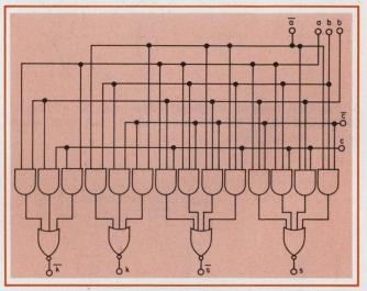
4. The single-bit adder implemented with two-rail AND-OR-INVERT logic. This configuration requires 14 AND gates, with each input driving six gates.
