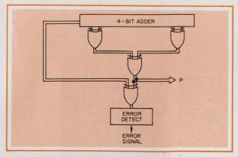
8. Sum and carry outputs of the four-bit adder are fed into an EXCLUSIVE-OR tree for a complete error check. The P, or parity, output is obtained as a by-product.
