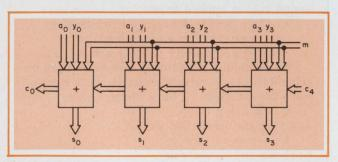
7. Four-bit adder/subtractor is formed by connecting four single-bit stages.
