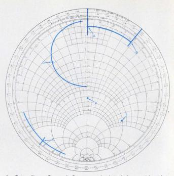
3. Capacitors  $C_{\rm s}$  and  $C_{\rm l}$  are calculated from this plot once the microstrip line length is fixed at 2.5 cm—a convenient value for our design. The capacitors for the remaining matching networks are determined in a similar manner.
