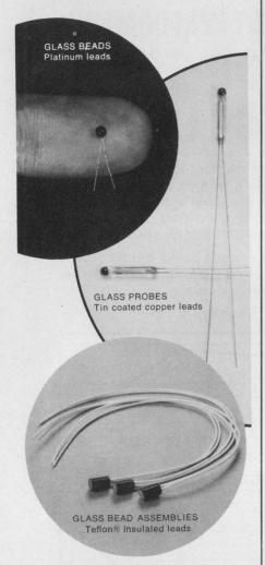
You can count on very fast response time and improved reliability even in hostile environments with Keystone's rugged glass beads, probes and assemblies. Select from a large range of resistance values (1 K to 1 meg at 25°C) and temperature levels from -50°C to 260°C. Easy to handle and assemble, these thermistors are ideal for temperature measurement and liquid level detection. Send now for data bulletin. Keystone Carbon Company, Thermistor Division, St. Marys, Pa. 15857.
