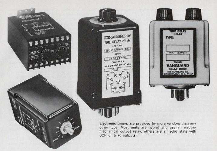
and first-cycle effects don't have their equivalents in pneumatic timers. Though some or all of these prob'ems can be solved in electronic units by special circuits and protectors, many users in the conservative machine-tool industry and in industries making industrial controls choose to stay with old reliables.
