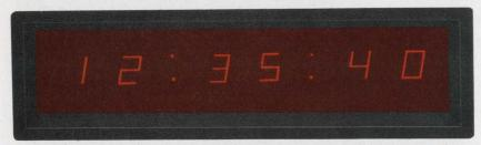
MAN1 — The standard of the industry, the .27" MAN1 is mounted on a 14-pin DIP and encapsulated in clear epoxy. Directly compatible with IC's, it is being used in a wide variety of alphanumeric display sockets. (Shown in a demonstration clock face.)
