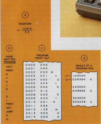
2. An equation containing transcendental functions like natural logarithms is easily programmed on an algebraic calculator. Enter variable x and answer y appears.
