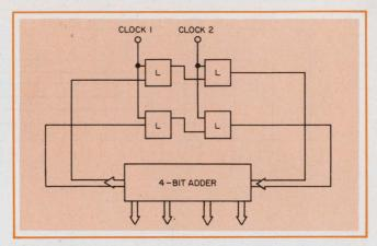
9. Two-rail latch pairs, connected as shown, are needed to delay the input carry with systems that use serial data transfer and two-phase clocks.
