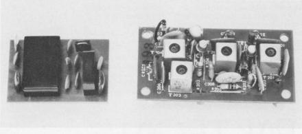
An integrated sound i-f detector using Semicon L (left) will be used to replace the more conventional discrete version (right) now used in television sets. The advantages include smaller size and fewer external components.
