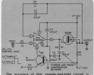
The accuracy of this sample-and-hold circuit is boosted by an operational transconductance amplifier and a MOSFET.
