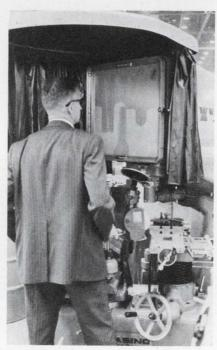
An optical projection profile grinding machine, built by Wasino Machine Co., Ltd., Nagoya, Japan, projects the grinding operation 25 to 50 times normal size. Wheels for grinding are directly below the projection screen.
