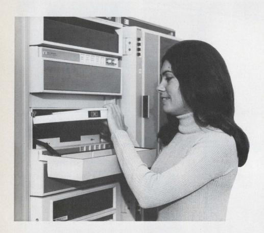
If you are an original equipment manufacturer in search of a low-cost high-quality memory for compact disc operating systems, HP has the answer. The new 7901A is a small, random-access moving-head disc drive with front loading, interchangeable cartridge and high-speed performance. The data capacity is 24 million bits with unlimited off-line storage.
