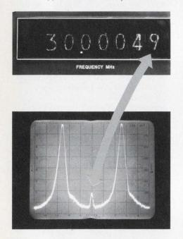
The modern spectrum analyzeralready eminently useful in lab, production and field applicationsbecomes significantly more powerful when coupled with a tracking generator. The combination can be used for precise frequency measurements of very low level signals and extremely wide dynamic range swept measurements of networks and devices. A new application note on tracking generator/ spectrum analyzer applications gives many examples, including specific setups. Check Q on the HP Reply Card for
