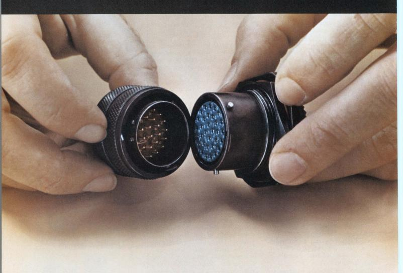
You know the bends. That's when connector pins are bent or damaged during mating by misaligned plug and receptacle.
