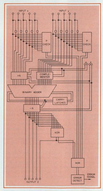
13. The complete binary/BCD adder/subtractor. Failures in either the inputs or the network are detected at the output of the single error detector.
