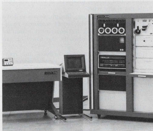
Tektronix's entry into the big-system market is the S-3260, which includes a graphic terminal among its standard features.
