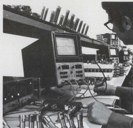
In a typical production test application, the 8755L large screen display shows forward- and return-loss response of components.
