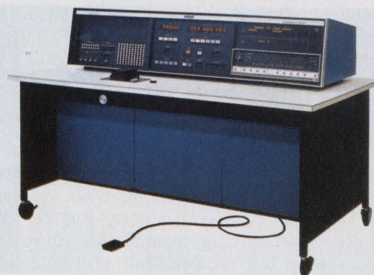
The Model 4400, which Datatron says was the first system to use force/monitor circuitry at each device pin.
