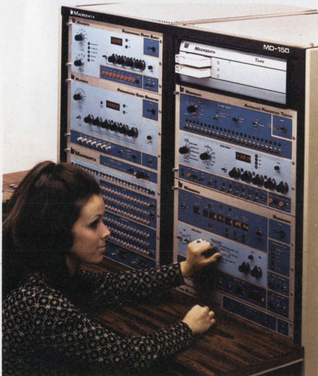
Macrodata's answer to obsolescence is the MD-150, a tester that features independent modules that can be replaced as necessary to update the system.
