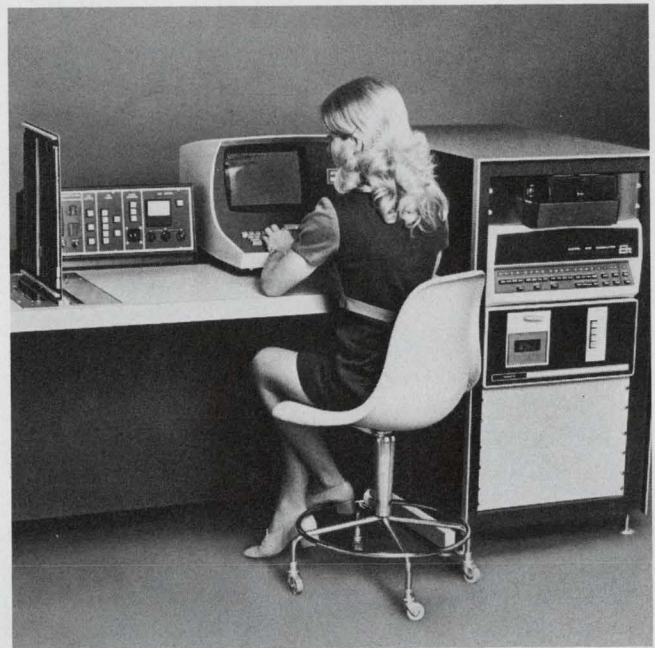
Computer Automation's Capable II uses the company's own 16-bit minicomputer. The system isolates faults in logic cards and IC devices.
