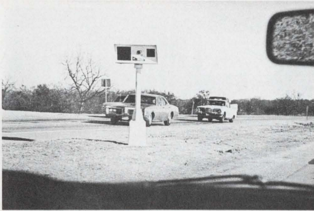
A new concept in traffic surveillance, ORBIS III, (left) automatically identifies a car, license number and driver and records vehicle speed, location, time and date on a
