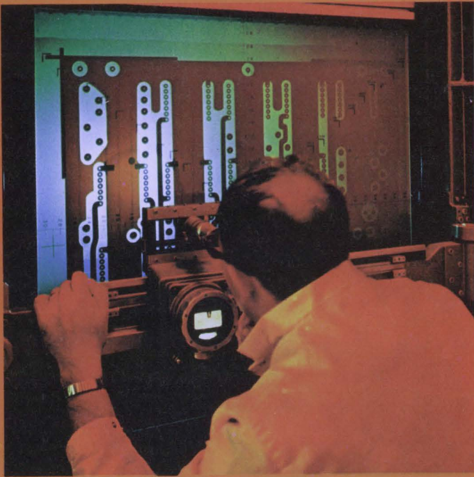
A restful red light is helpful to the operator who must look into green light on this Dainippon 59 reduction camera.
