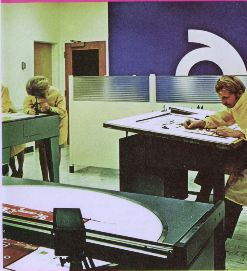
Graphic artwork specialists prepare high-precision multilayer printed circuit card artwork. White "A" on blue wall stands for "artwork." The red line ending in a bull's eye leads the eye into the room from the supervisor's office.
