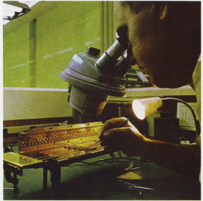
Technician at Sperry Rand Univac inspects diode modules on a plated wire aerospace memory plane. LSI will spur development of ever smaller memories.
