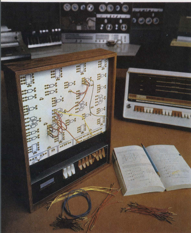
Students can learn digital logic and computer fundamentals by correctly connecting patchcords in Digital Equipment Corp.'s "Computer Lab."
