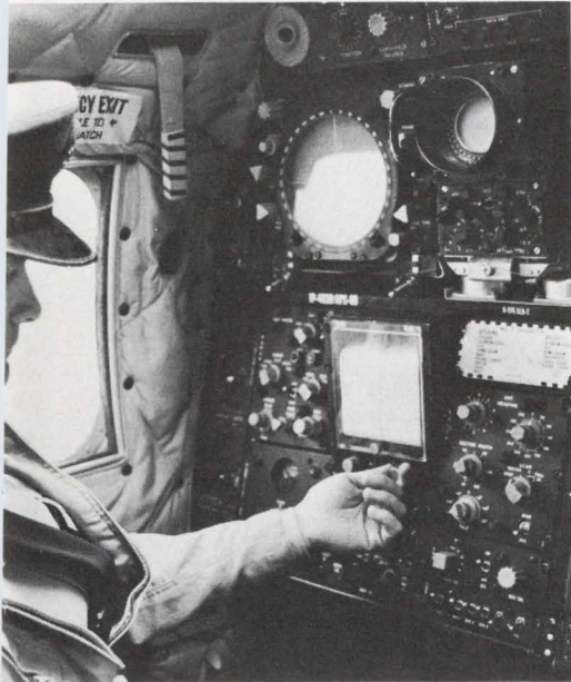
Operator in S-2E carrier-based patrol plane looks at magnetic anomaly detector display below radar scope. ECM is upper right.
