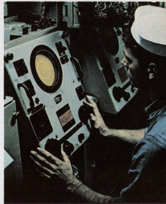
Operator tests AN/SQS-30 hull-mounted, active sonar aboard destroyer Borie. Far scope is for variable-depth sonar.
