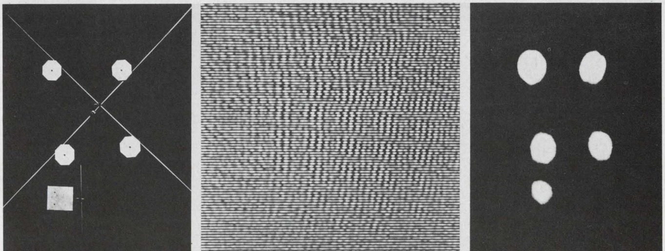
Acoustic hologram of array of aluminum panels is formed by detecting ultrasonic waves that reflect from their surfaces. Raster scanning causes the horizontal bands,
