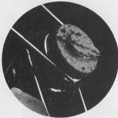
Brush assembly of conventional synchro after 1000 hours
