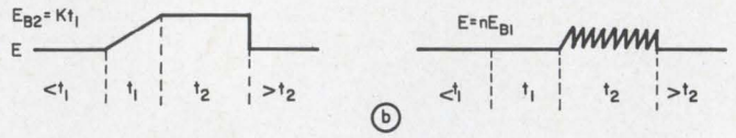
2. Ratio computer circuit is used to determine ratio of t_2:t_1 , which is proportional to the number of input pulses.
