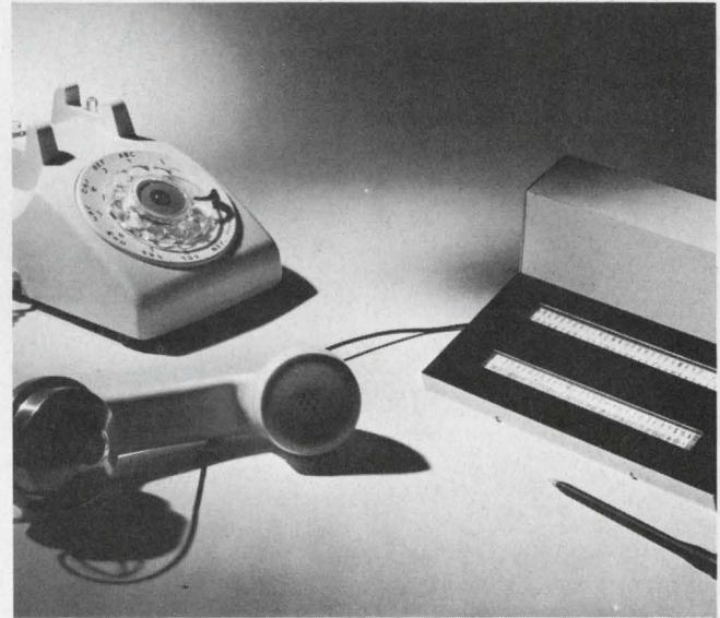
Portable electronic keyboard allows computer data to be fed in over telephone lines. Page 34
