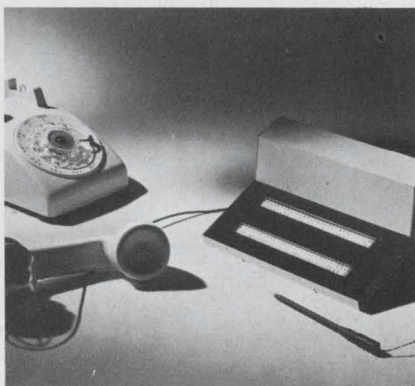
Computer input-output device can be carried around and plugged into any telephone.
